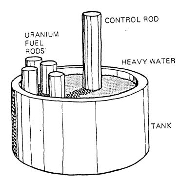
Figure 5 The zero-power reactor experiment
