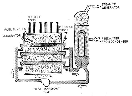
Figure 6 The CANDU power reactor experiment
